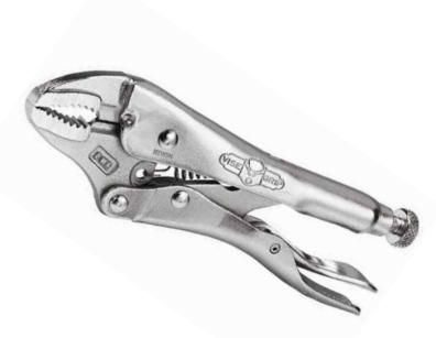
VISE GRIPS are essentially pliers that can be locked into place and are a versatile gripping tool. They have a bolt at the end of one of the handles which is used to adjust the opening size of the jaws, and a lever on the other handle to release the jaws once they are locked. Vise Grips are available in many different shapes and sizes, including needle nose and locking clamps. They can function as pliers, clamps or in place of wrenches in many cases.
